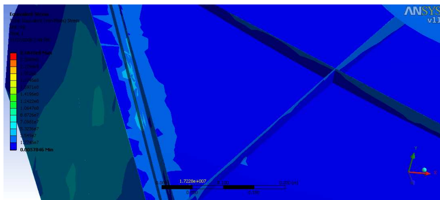
Figure 12.18: FM2-MKVI cross section of stresses during torsion test
