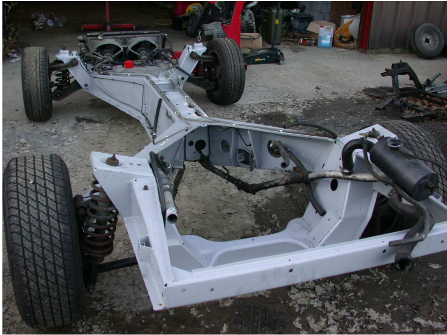
Figure 7.1: Delorean backbone chassis
